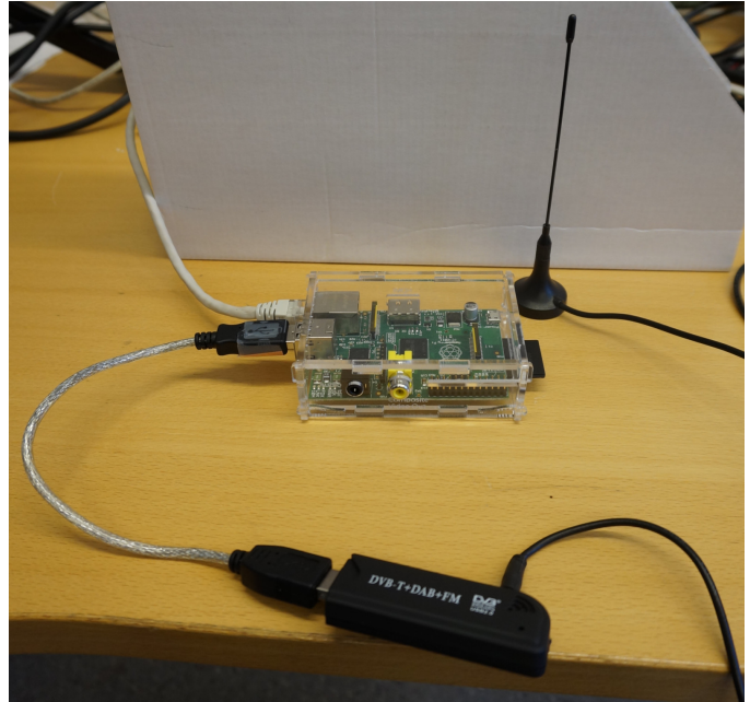
Figure 2: A Raspberry Pi-based sensor node, with SDR capable USB dongle attached.
